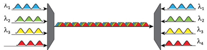
Figure 6: SWDM combining four wavelengths from 850 nm to 940 nm
