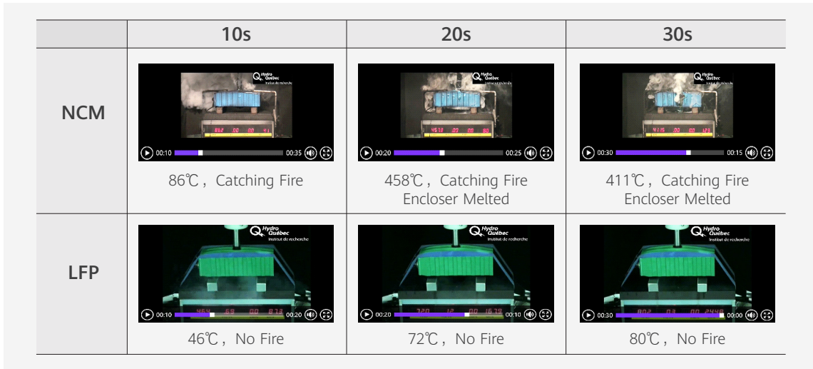
Figure 6: Safety test comparison between LFP and NCM batteries (puncture test)
