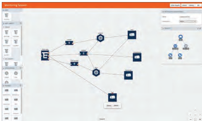
Figure 4-6: The NGNPB orchestration and management module can manage policies for monitoring network traffic on the cloud platform. (Source: Gigamon)
