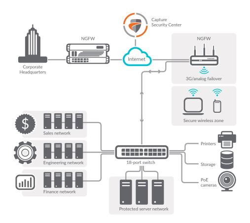
**The workhorse of network security.** Firewalls serve as the backbone to many security deployments. In this example, an enterprise uses next-generation firewalls to protect a wide range of assets, including endpoints, remote networks and locations, servers, IoT devices and more.
