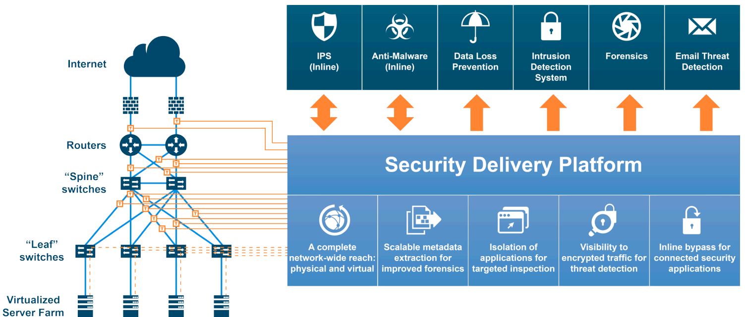
Figure 4: A Security Delivery Platform: Key components
