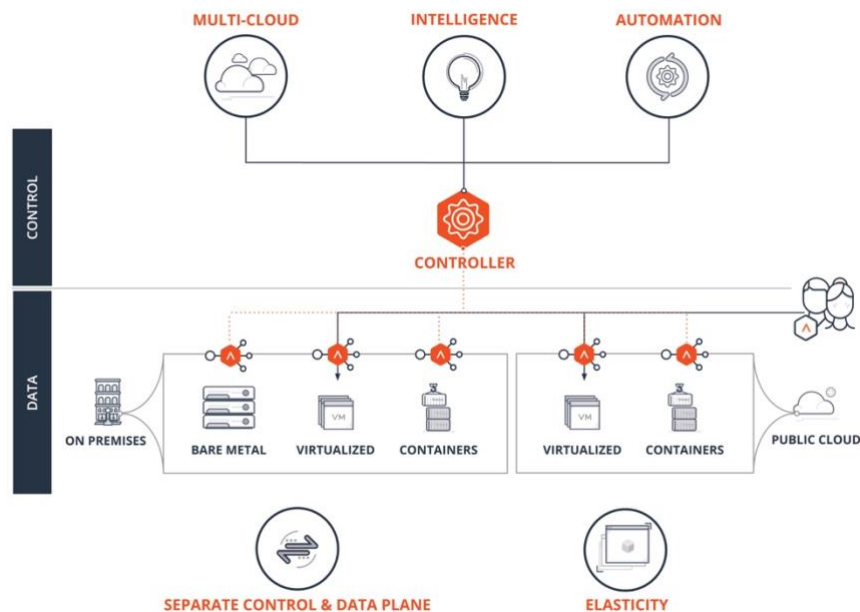
Figure 2: NSX Advanced Load Balancer – high-level architecture
