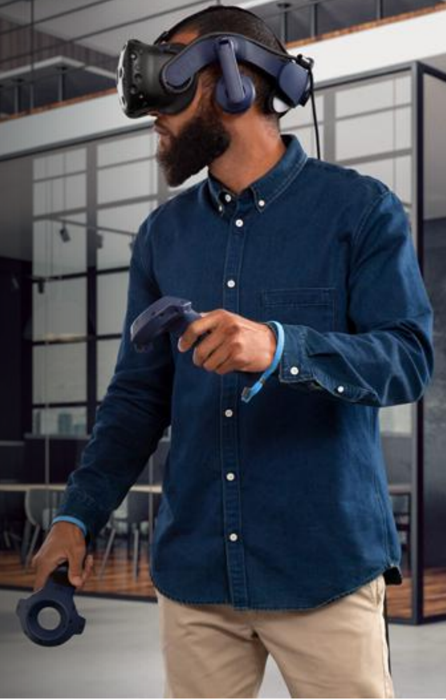
HTC Vive Pro 2 Visualize in 5K fidelity. Explore VR content in brilliant clarity and bring out the finer details with a combined 4896 x 2448 resolution.
