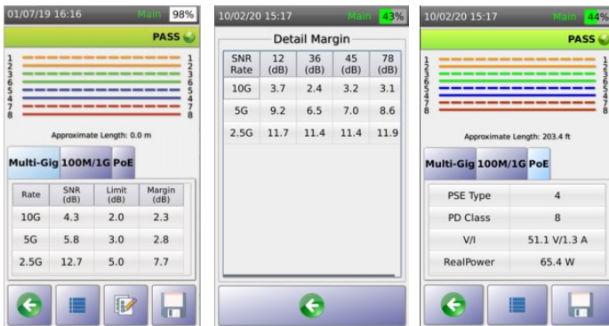
Fig 4 : SNR based link speed measurement while under traffic and PoE load
