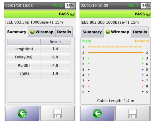
Fig 16 : Single Pair Ethernet (SPE) cable integrity assurance
