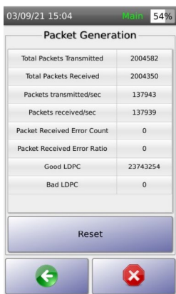
Fig 12 : Example of quick and simple packet generation function
